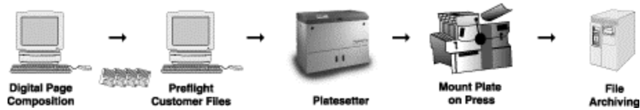
Figure 2: H. C. Miller's Computer-to-Plate Workflow
